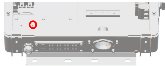
Fig. 22: Potential equalization (Decentral ConnectionBox)
