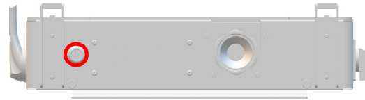
Fig. 26: Connection area: communication
